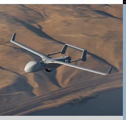
Integrator ER uses satellite-enabled communications (SATCOM) to extend flight range beyond line of sight (BLOS), expanding target sets, reducing the logistical footprint and enhancing personnel safety.
